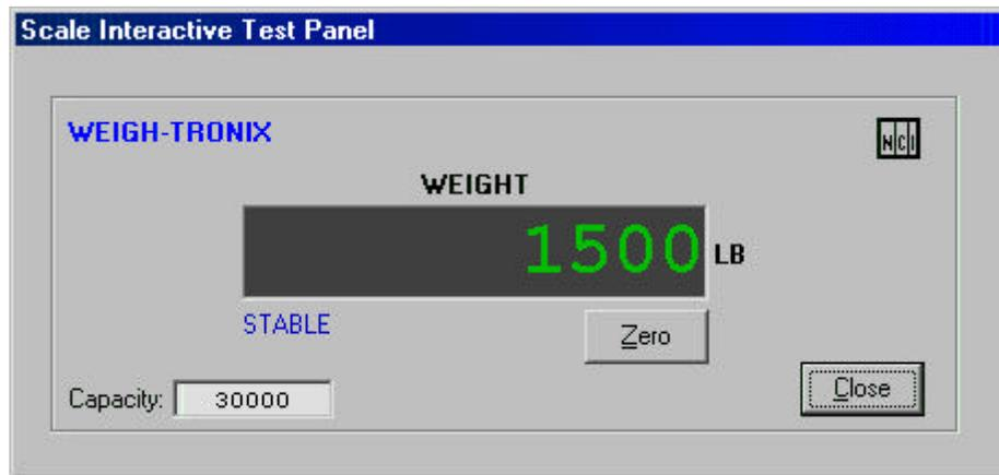
In operation, the panel will dynamically display the current weight on the scale with its units-of-measure. In addition, it will indicate whether the weight is **STABLE** (or not) and error conditions **OVER CAPACITY** or **UNDER CAPACITY** (if/when applicable).
